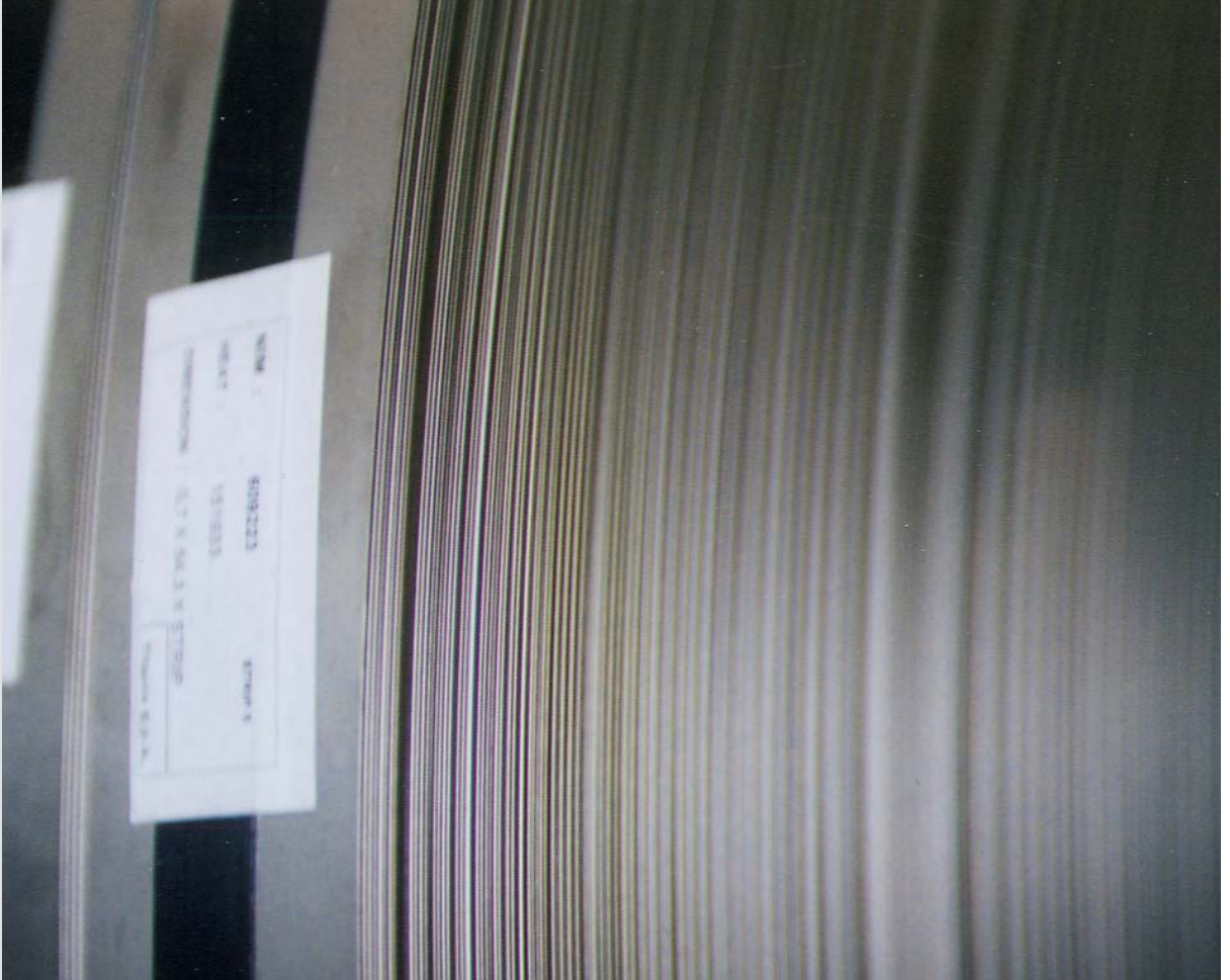
Titanium sheet | The coils rolled at ThyssenKrupp Acciai Speciali Terni are cut into 30 to 120 millimeter wide strips at the C.S. Inox service center. The strips are then laser welded into tubes at Titania. Photo: Rainer Kaysers
