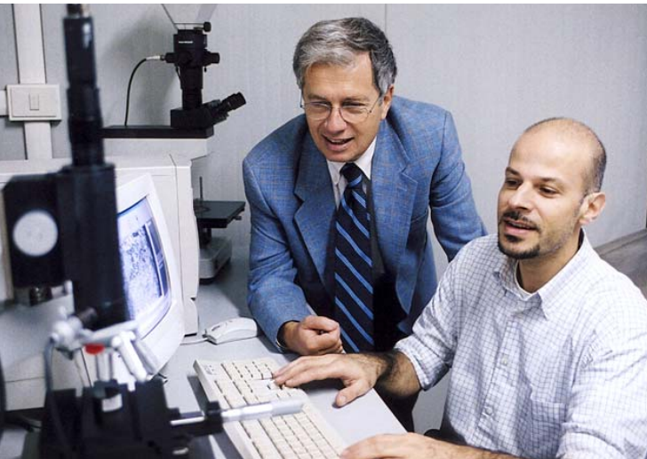
High-tech | Research chief Fabio Guglielmi (left) and Sergio Cervo check the microstructure of the tube welds to ensure they meet the specifications for seawater desalination plants. Photos: Rainer Kayzers
